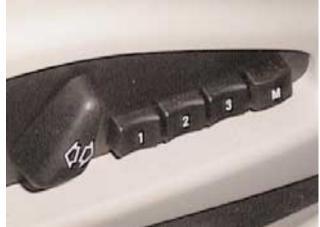
The stored position can be recalled at any time by pressing the appropriate memory location button (1-2-3).
